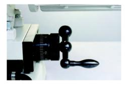
Setting the gap width between the two grinding disks is carried out by simply adjusting the rotary handle attached below the drive motor with scaling (1 graduation mark - 0.02 mm).
