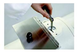
With a feeler gauge (if unavailable normal printer paper that has been folded once can also be used), set the gap to 0.1 mm using the rotary handle.
