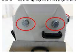
**1.** Loosen the fastening screws (fastening nuts for ZrO<sub>2</sub>) with a 30 mm spanner before opening the grinding chamber.
