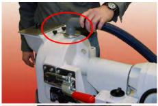
After a grinding process has ended, you can suck off the dust that has accumulated during grinding, by attaching the vacuum cleaner connection piece (order no.: 13.1450.00) to the window in the grinding chamber (checking the gap adjustment). Assemble the connection piece and the vacuum cleaner exhaust hose as shown in the images.
