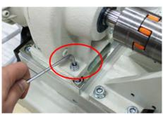
**4.** Remove the motor fastening screw under the oil drain screw with a no. 6 hexagon socket screw key.
