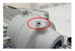
The gears of the motor are filled with gear oil at delivery (ISO VG 220 Ord. no.: 85.0110.00). To change the gear oil, there is an unscrewable filler screw at the top of the gear housing.
