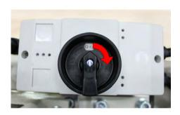
Switch main switch (10) to ON (I). The disk mill starts up.
