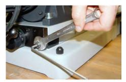
Turn the stop screw back by using a 4 mm hexagon socket screw key to turn it to the left (max. 2 turns).
