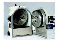
The comminution of the material sample is done in a grinding chamber, which is sealed dust-proof to the outside, in which two roughly meshed grinding disks work against each other. The movable grinding disk is driven by a powerful, slowly running gear motor. (Depending on the voltage, 421 - 505 rpm, see & Chapter 3.7 'Speed' on page 15)
